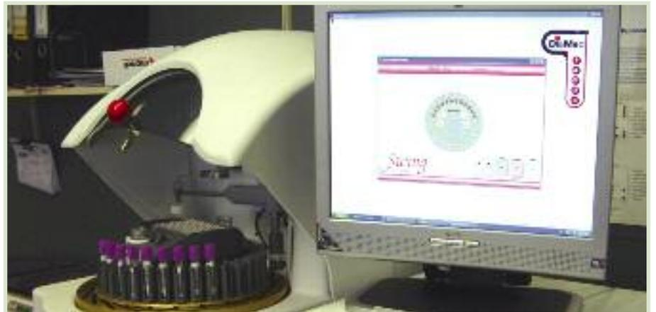
Fig. 1 DIAMED SWING used at Clinipath Pathology for automated blood grouping and antibody screening
